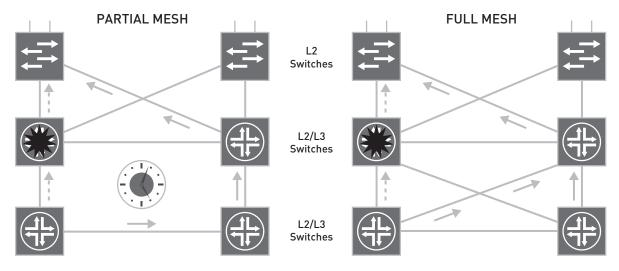
Figure 8: Full mesh versus partial mesh connectivity
