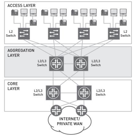
Figure 4: Aggregation layer in a highly available campus LAN
