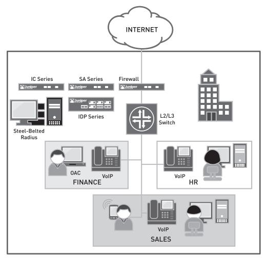
Figure 10: Security architecture in a campus environment
