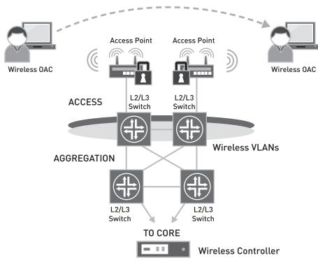
Figure 3: Flexible and roaming wireless access solutions
