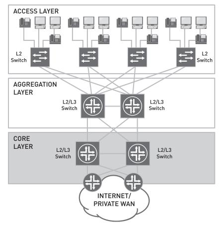
Figure 5: Core layer in a highly available campus LAN
